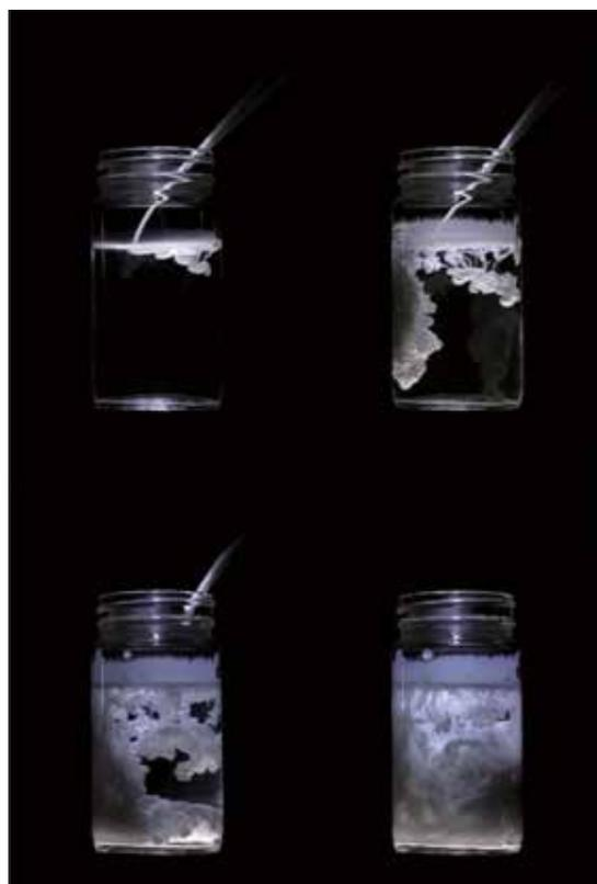
**Figure 3: Blooming effect of Azoxystrobin 250 SC upon dilution**
